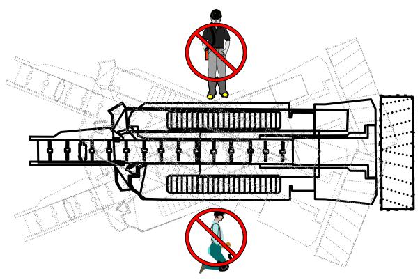
Many miners believe that the pivot point of the continuous miner is a safe place to position themselves. The pivot point is within an unsafe area, or Red Zone. The continuous miner is not a stationary piece of equipment, and the pivot point moves as the machine moves. Also, unintentional movement of the machine is possible as conditions change. Miner operators must protect themselves and their coworkers from unintentional movement, mechanical problems, and human error.
